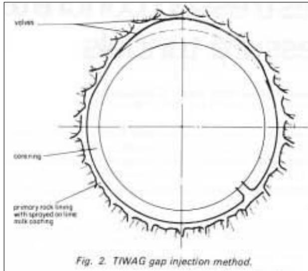
Fig. 2. TIWAG gap injection method.
