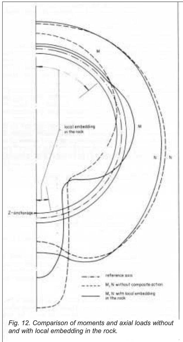
Fig. 12. Comparison of moments and axial loads without and with local embedment in the rock.
