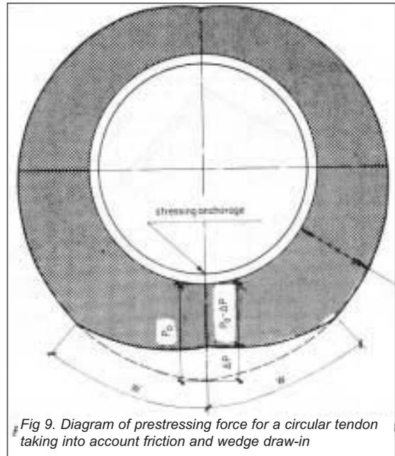
Fig 9. Diagram of prestressing force for a circular tendon taking into account friction and wedge draw-in
