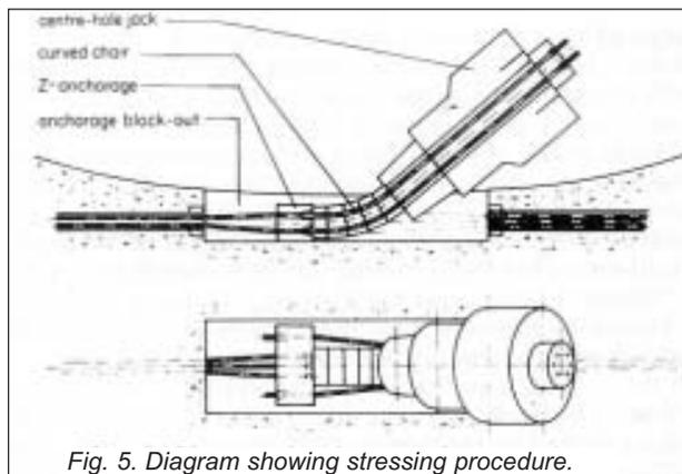
Fig. 5. Diagram showing stressing procedure.
