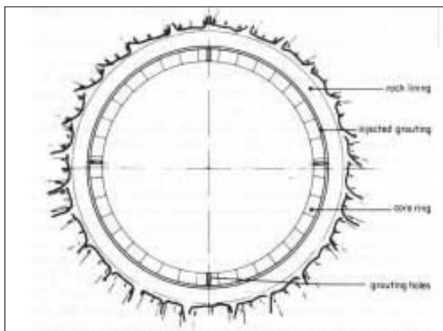
Fig 1. Core ring lining by the Kieser method. Construction with core ring of blocks.
