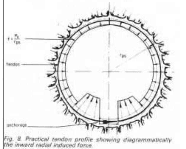
Fig. 8. Practical tendon profile showing diagrammatically the inward radial induced force.
